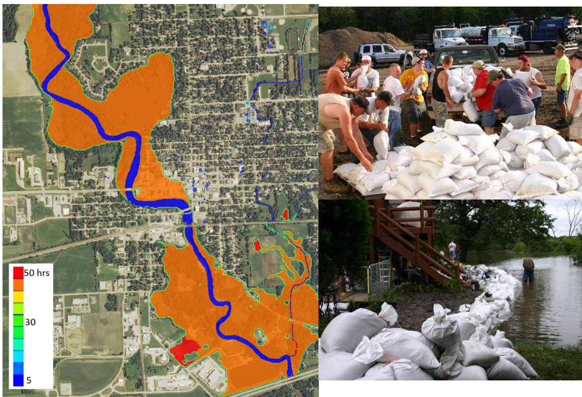
Figure 47. XP-C2 IFC time to peak water surface elevation (hr) for the July 2010 event compared to photo
